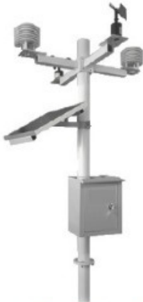
Automatic Weather Station
